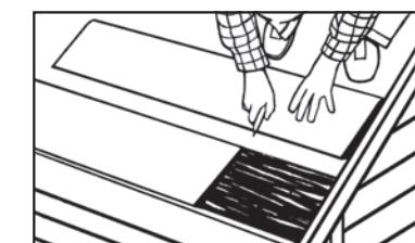
Step 4 – Use utility knife to cut final section to length. Integrated end plug of final section should be flush with end of roof. Pre-fasten final section.
