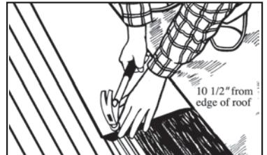
Step 3 – Making sure the slot is open from step #2, position the Intake Vent over venting slots. Make sure that the lower edge of the venting is aligned with the edge flashing. Start at end of roof so that end plug is flush with end. Locating tabs on underside of the Intake Vent may assist in positioning over slot. Use reinforced nail holes to pre-fasten vent in place.
