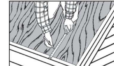
Step 1 – Remove all roofing materials for reroof applications. Install edge flashing and gutter straps as necessary. Measure 5" from edge flashing bend to mark lower slot line. Measure 3/4" further up to mark upper slot line.
