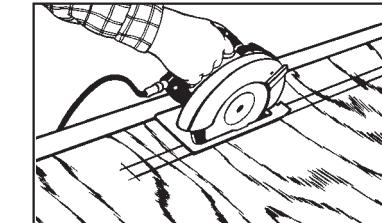
Step 2 – Install either felt (warm weather climates) or WinterGuard™ waterproofing shingle underlayment (cold weather climates) onto the bare deck 10-1/2" from the edge of roof up the slope. Cut slot with circular saw. Warning: Adjust depth of blade to avoid cutting rafters or trusses. Refer to drawings above for slot dimensions. Remove debris from slot.
