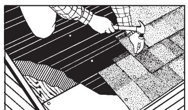
Step 6 – Install starter and first course shingles over felt/WinterGuard™ waterproofing shingle underlayment-covered Intake Vent using shingle manufacturer guidelines for shingle overhang and nailing requirements. Nailing patterns may have to deviate from some shingle installation instructions to avoid nailing in slot location.
