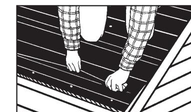
Step 5 – Install either felt (warm weather climates) or WinterGuard™ waterproofing shingle underlayment (cold weather climates) over The Intake Vent being careful to avoid nailing into the roof deck slot. Using a chalk line, transfer the nail line (2-5/8" from drip edge) and slot location (5-3/4" to 7" from drip edge) to the top of the felt or WinterGuard™ waterproofing shingle underlayment.
