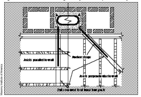
Figure 3. Two methods for securing chimney anchor straps to wooden joists.
