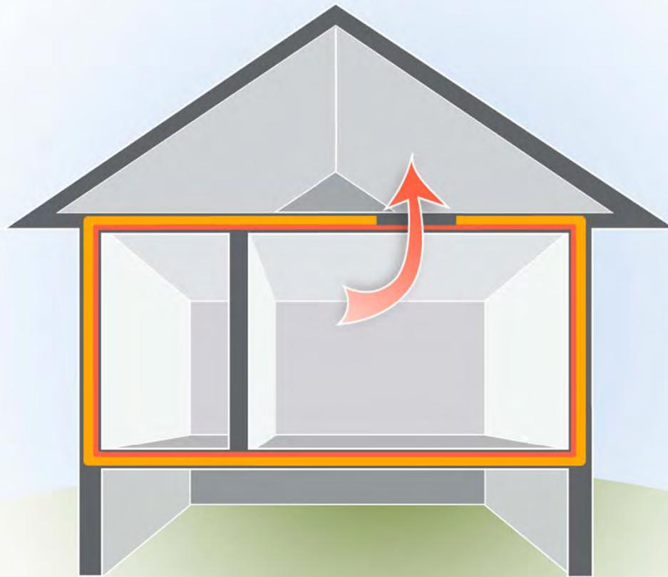
An uninsulated attic hatch is a gap in the attic's thermal barrier.
