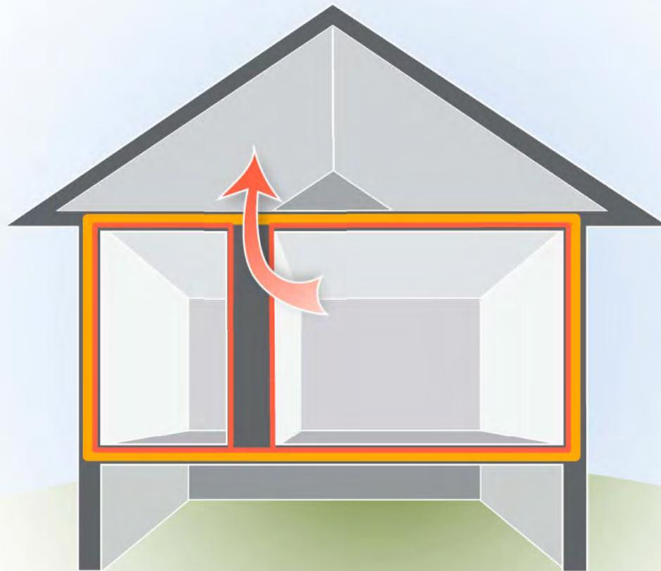
A mechanical chase containing ducts can break the attic's air barrier.
