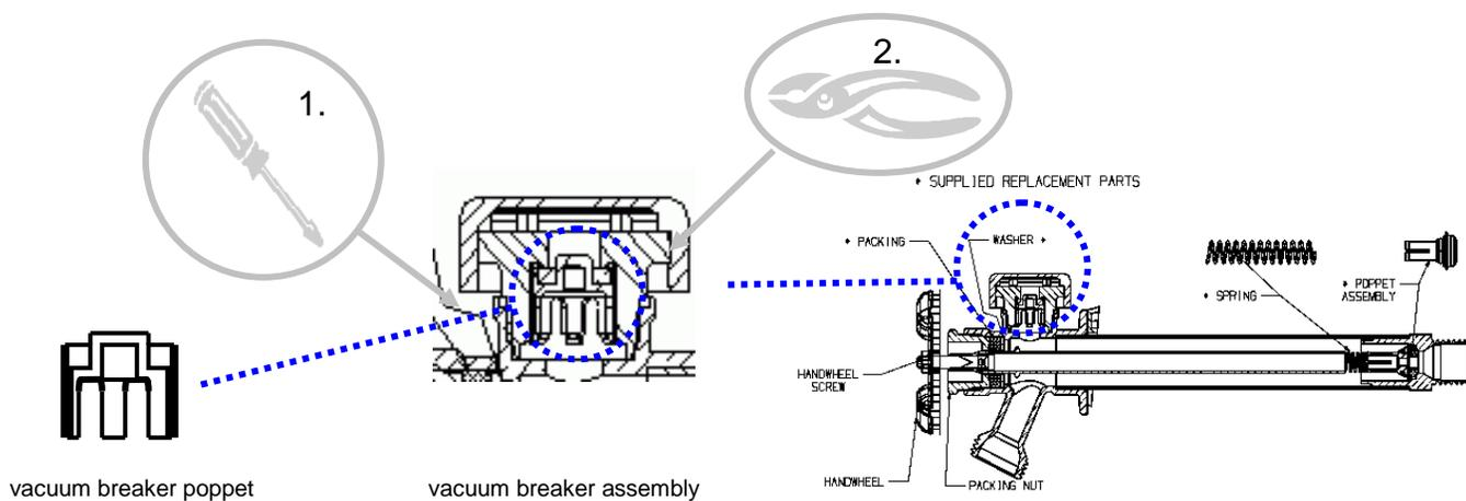
The NIBCO Figure 90 Frostproof valve (sometimes referred to as a sillcock or hydrant) employs an integral vacuum breaker. The vacuum breaker's function is to prevent any potential siphon effect (via a connected garden hose) in the event of a significant drop in line pressure, thus preventing undesired backflow that could draw contaminants into the potable water supply.
