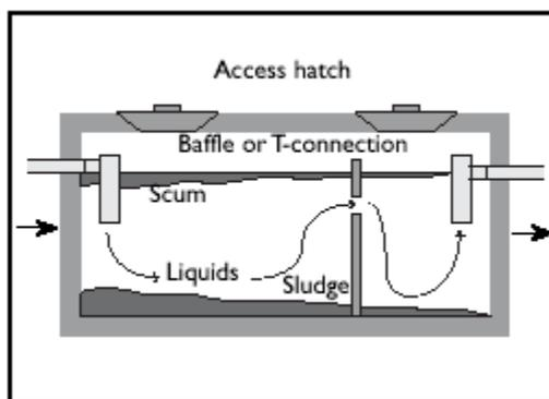
**Figure 4: Common Septic Tank (source: CMHC)**
