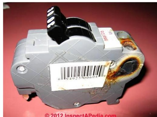
**Fig. 7. Burned-Out GTE Sylvania Zinsco™ Circuit Breaker.**
