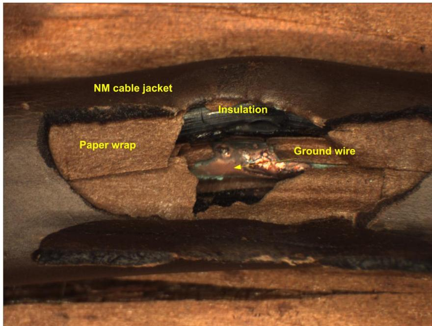
Figure 48 - Arcing area of damaged NM cable
