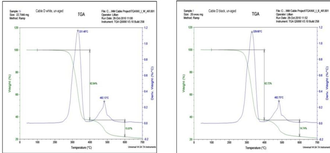
Figure 7 - TGA from Cable D Insulation
