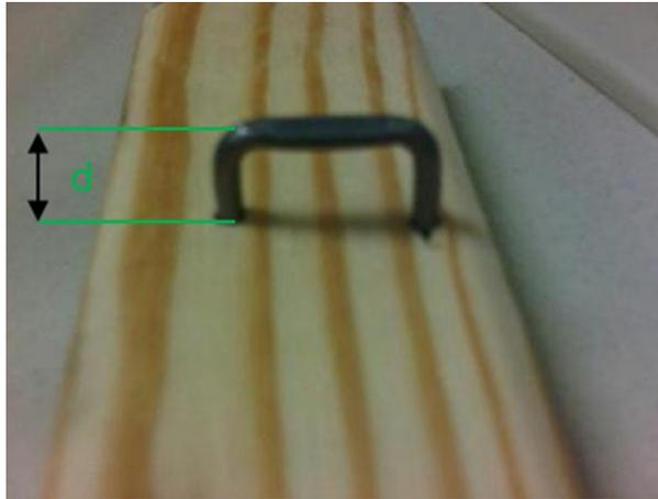
Figure 25 – Illustration of staple depth by hammer blows
