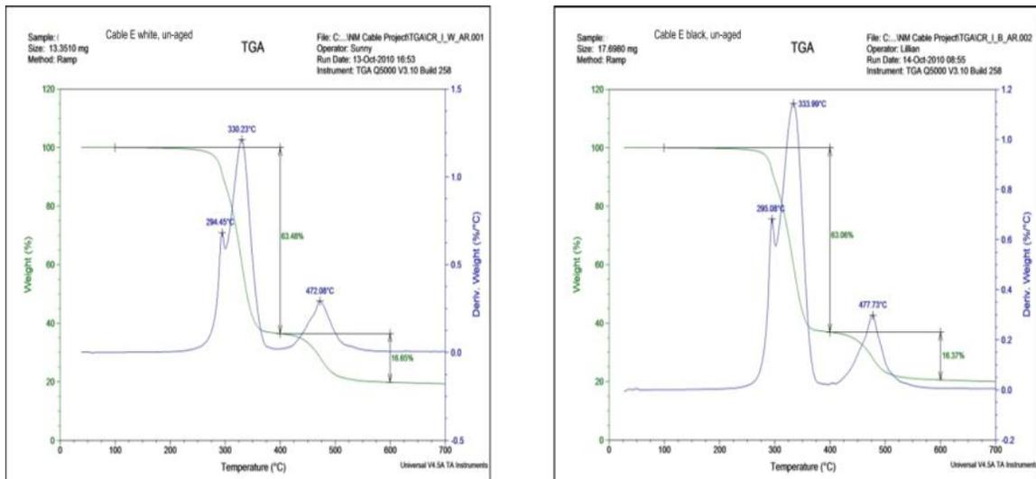
Figure 8 - TGA from Cable E Insulation
