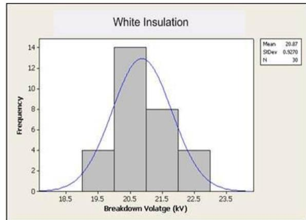
Figure 17 - Cable D breakdown voltage distribution
