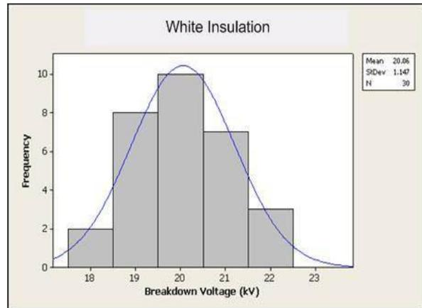
Figure 14 - Cable A breakdown voltage distribution
