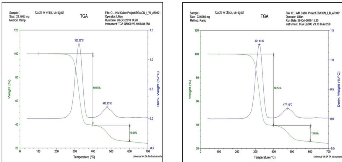
Figure 4 - TGA from Cable A Insulation
