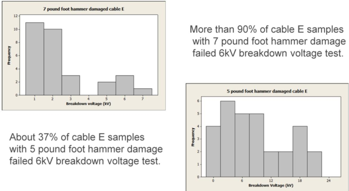
Figure 32 - Breakdown voltage distribution of cable E damaged by hammer impact
