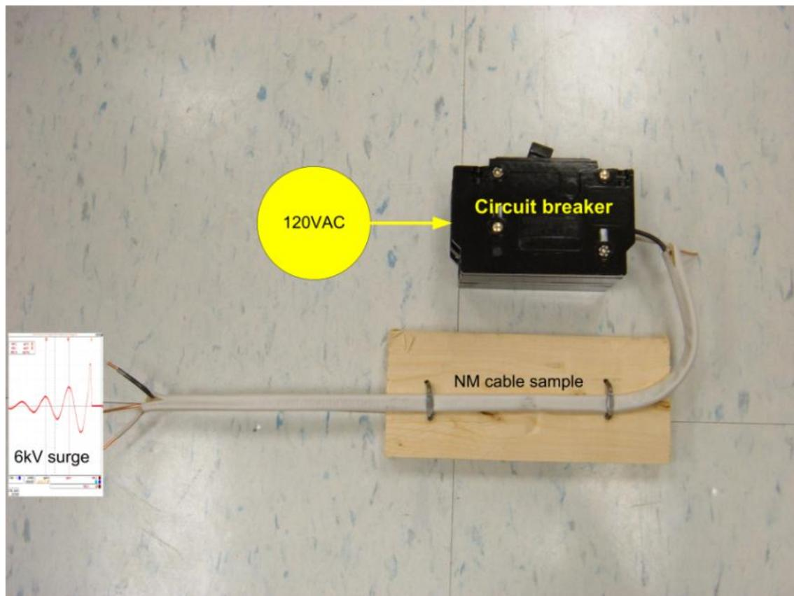
Figure 46 – NM cable voltage surge test schematic.
