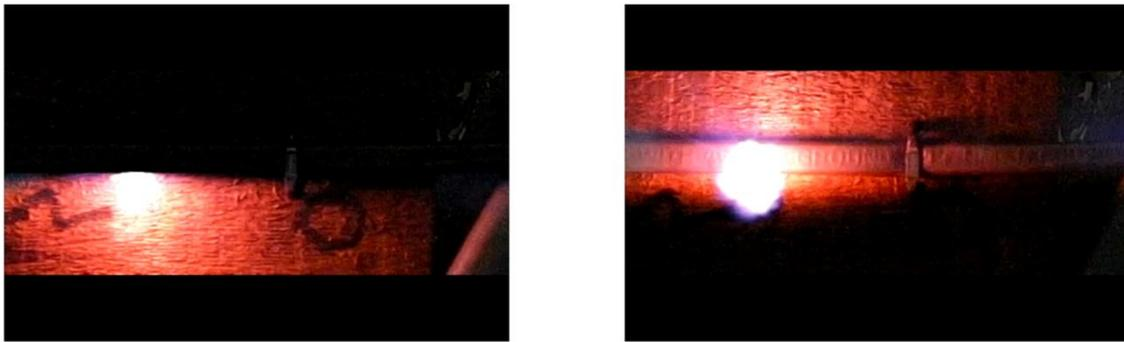
Figure 47 – Voltage surge generated electrical arc. On the left is the 1<sup>st</sup> image with arc, on the right is the 2<sup>nd</sup> image with arc.
