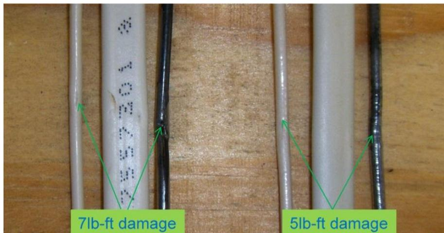
Figure 29 - Comparison of 7ft-lb and 5ft-lb damaged NM cable samples
