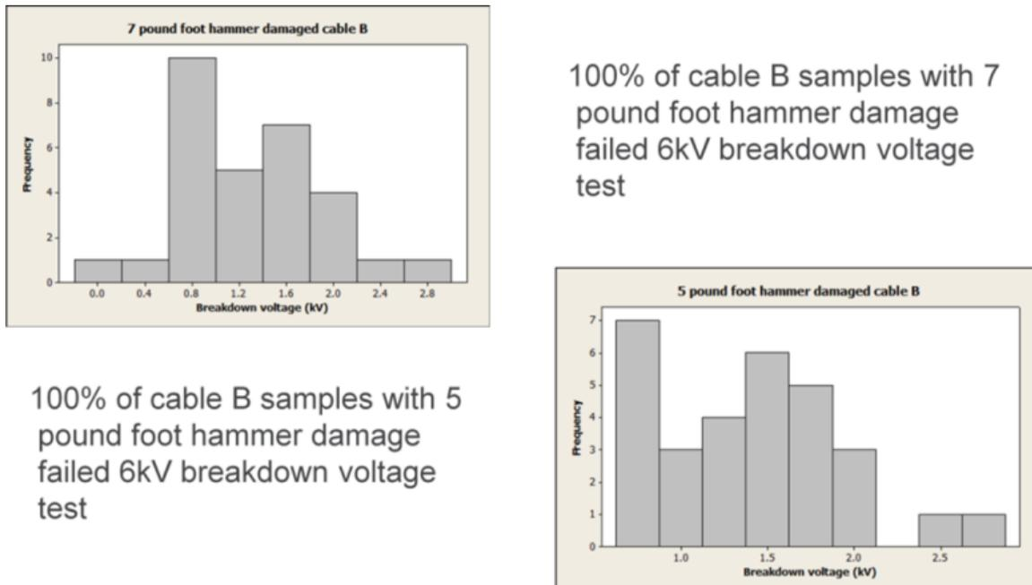
Figure 33 - Breakdown voltage distribution of cable B damaged by hammer impact
