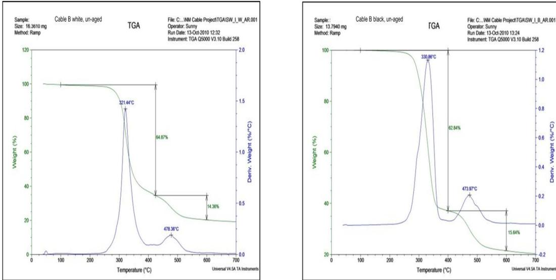
Figure 5 - TGA from Cable B Insulation
