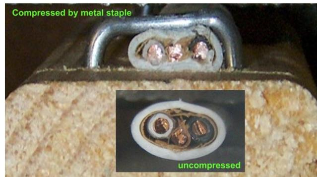
Figure 23 - NM cable compressed by a metal staple
