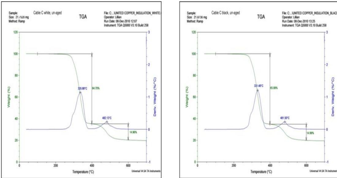
Figure 6 - TGA from Cable C Insulation
